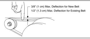
Fig. 33 Check Belt Tension with Finger
